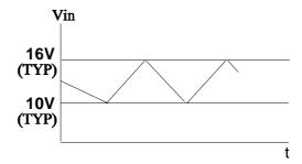
In this condition the  $V_{\rm IN}$  terminal pin 4 decreases until the shutdown voltage of 10V is reached. At this point pin 4 begins to rise again but when it reaches the start up level of 16V, the latch circuit continues to stop the drive.
